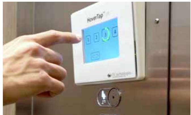
An early HoverTap prototype being used to select a floor in an elevator.
